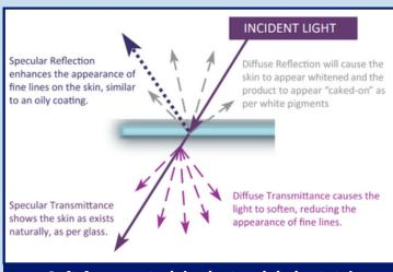
Soft-focus materials aim to minimize total reflection as well as maximize diffuse transmittance and total transmittance.
